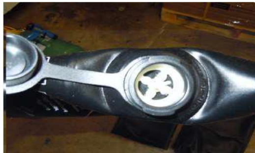
Air bag valve: Turn white stem until it pops up and seals closed. Stem rotates open & closed.
