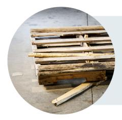
Recycled wood pallets often failed in transit-resulting in damaged POP displays, disrupted setups, scratched store floors, and compensation claims from retailers.
